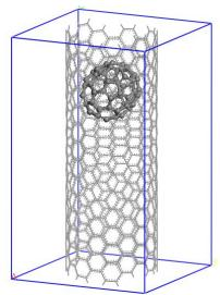
which consists of a  $C_{70}$  fullerene inside a single repeat-unit of a (10,8) carbon nanotube. The (10,8) is a chiral nanotube with 488 atoms in each repeat-unit, so the peapod input consists of 558 atoms, with no symmetry, in a unit cell of 20.0Å x 20.0Å x 33.27Å. The ONETEP input is in the file  $C_{70}in_{10-8.dat}$ . We impose a density kernel cut-off of 25.0 a<sub>0</sub> (KERNEL\_CUTOFF 25.0) in order to achieve linear-scaling behaviour.
